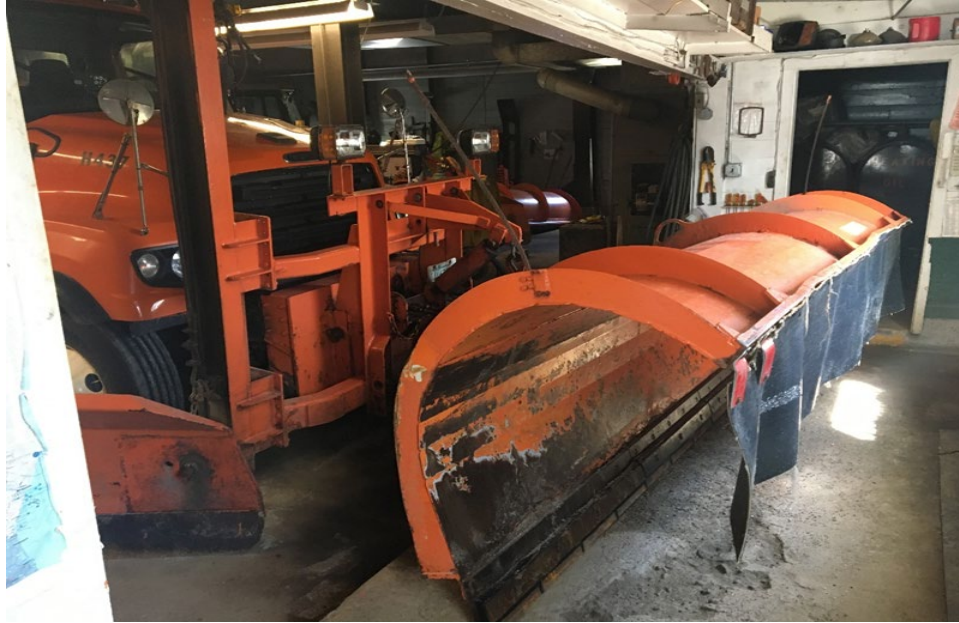
Photo-3: View of the front of truck with plow equipment mounted and parked in shed. Minimal clearances and uneven surfaces throughout the building make it difficult to navigate and increase risk of accidents and injuries.
