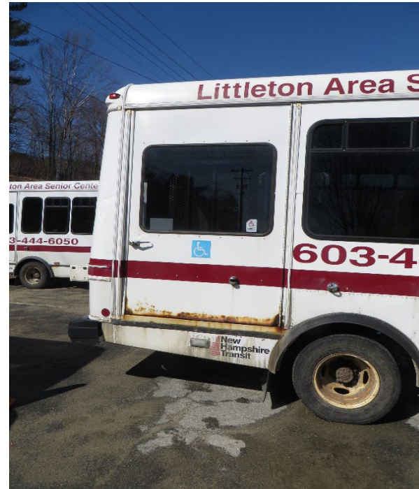
GCSCC: Corrosion on body panel
