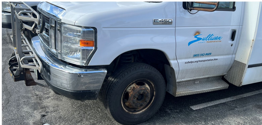
SCS: corrosion on wheel & running board
