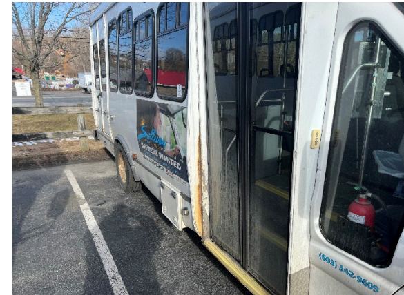
SCS: Corrosion on passenger door
